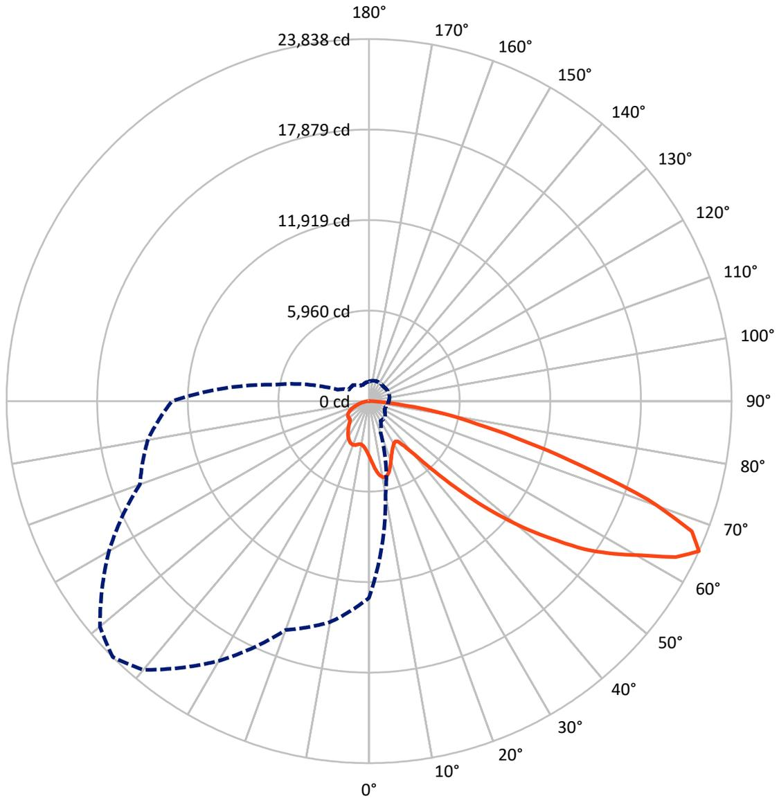
— Vertical Plane Through 315-Deg Lateral      - - - Horizontal Cone Through 65-Deg Vertical
