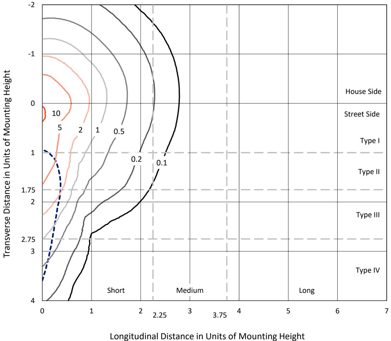
Based on 20 foot mounting height. Maximum calculated value = 10.9 fc
